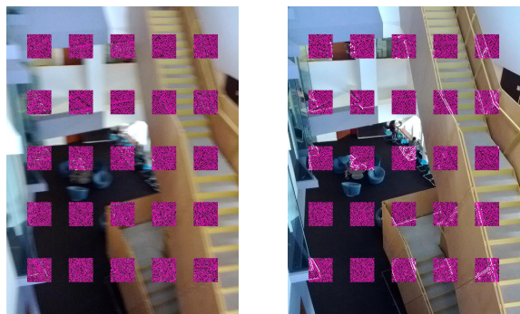
(a) Blurry (b) Sharp We apply a Sobel filter to 25 patches. Here, the resulting gradients are shown overlaid on the original image.
