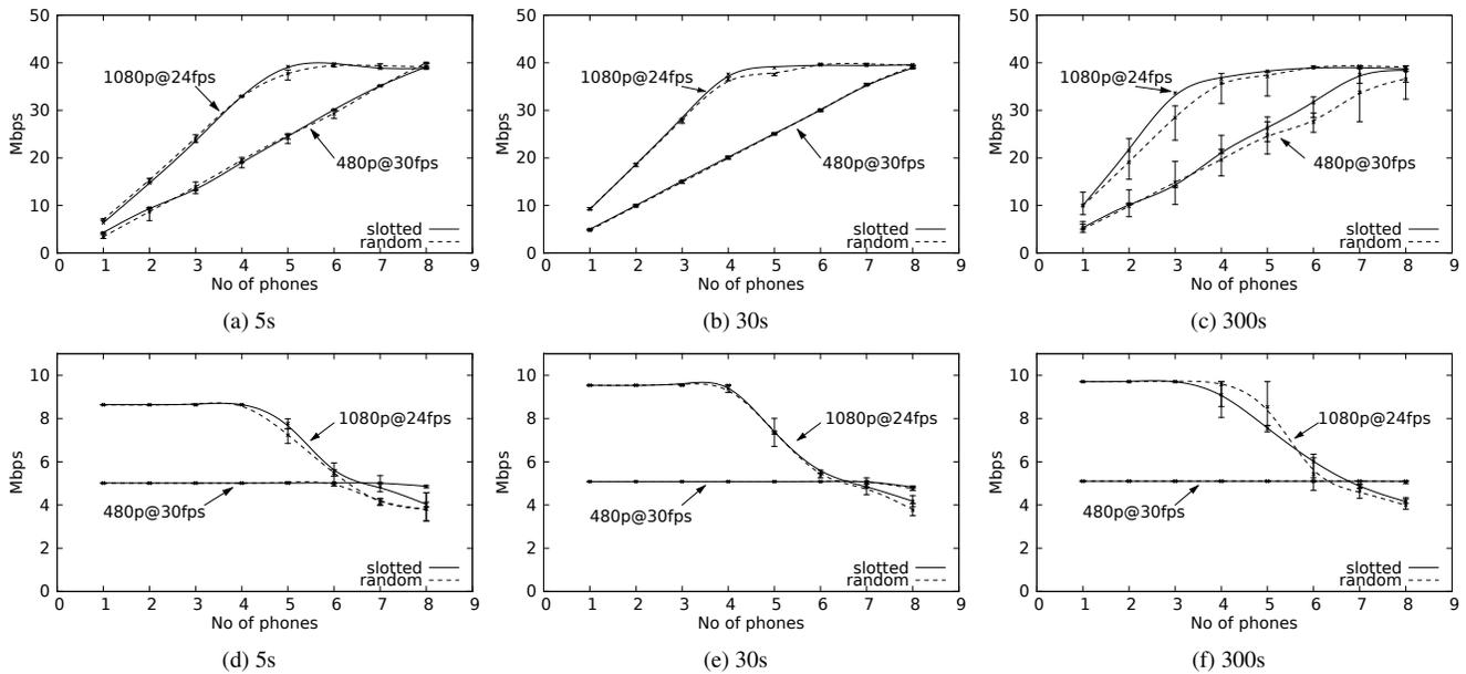
**Figure 7: Throughput [Mbps] for different resolutions and video framerates. The figures on the top row show the cumulative throughput of the AP, the bottom row shows the net throughput achieved by each phone.**
