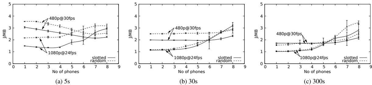
**Figure 8: Energy consumption of video upload from Nexus I9250 via 802.11n.**
