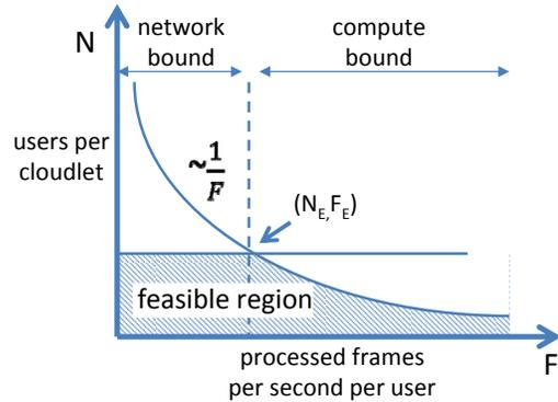
**Figure 13: Model of tradeoff between number of users ( $N$ ) and processed framerate per user ( $F$ ). The shaded region represents the range of feasible choices with fixed network and processing capacity.**
