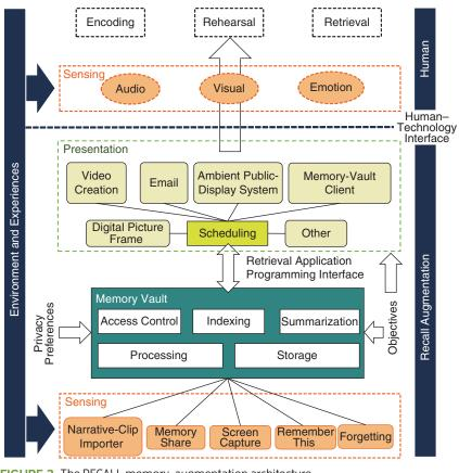
FIGURE 3. The RECALL memory-augmentation architecture.
